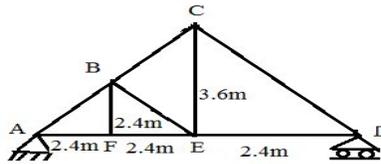
3. Find the forces in all the members of the girder shown in Fig. by the method of joints, indicating whether the force is compressive or tensile.
