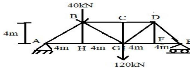
5. For the truss shown in fig find the forces in members CD, CB, BD and AE by method of joints.
