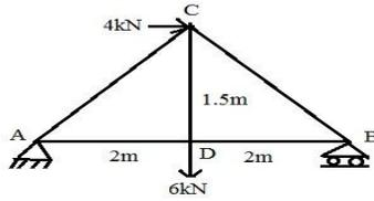
2. Find the forces in the member of the truss shown in fig. by method of sections.
