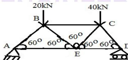
4. Determine the forces in all members of a truss as shown in fig.
