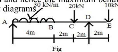
2. Draw the shear force and bending moment diagram for the beam shown in Fig. Indicate maximum positive bending moment and its location.
