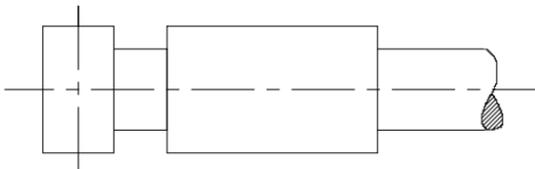
**Fig. 2.8 Full form cylindrical plug gauge**
