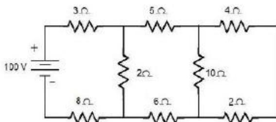
7. Calculate a) the equivalent resistances across the terminals of the supply, b) total current supplied by the source and c) power delivered to 16 ohm resistor in the circuit shown in figure. (16)
